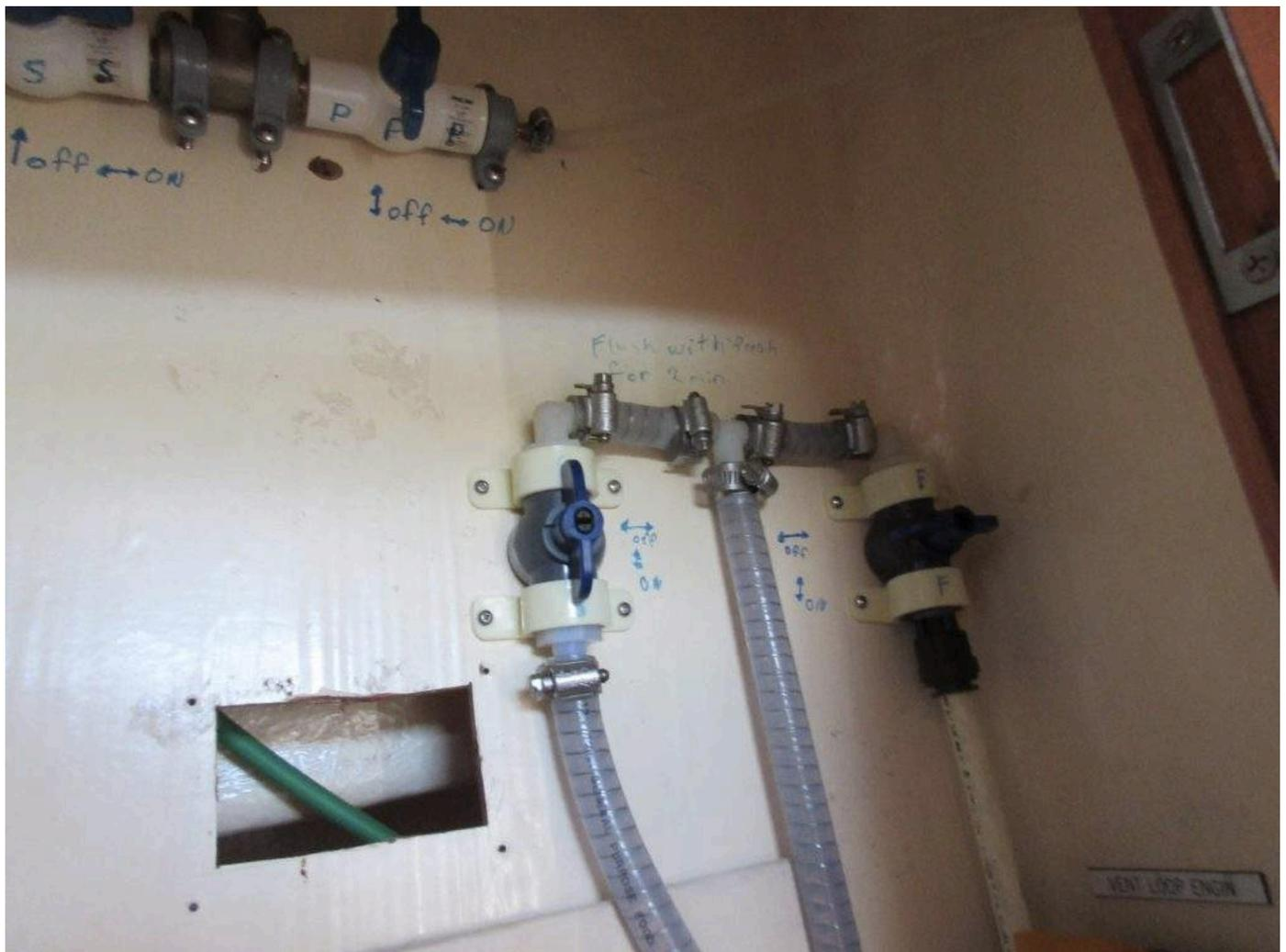
Although this looks confusing, it really isn't. The 2 lower valves are used for flushing and the 2 upper valves let me put water in starboard, port or both tanks. I really need to find a label maker and make it more professional!
