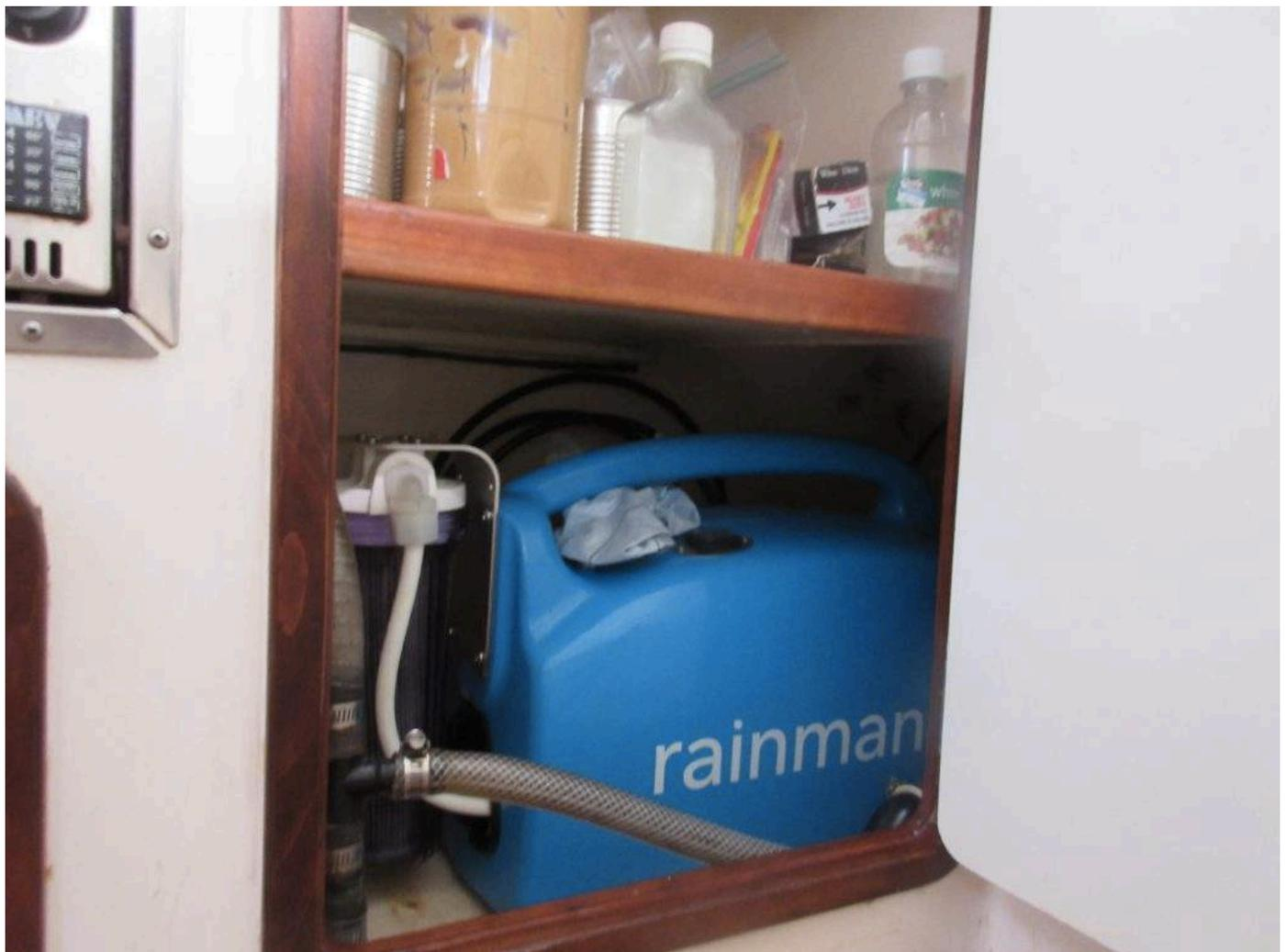
The pump unit fit perfectly in the location of the old watermaker membranes. All the hoses and cables were left long enough to allow us to pull it out for servicing the oil (there is a service hatch behind the unit and it pulls out in the closet).
