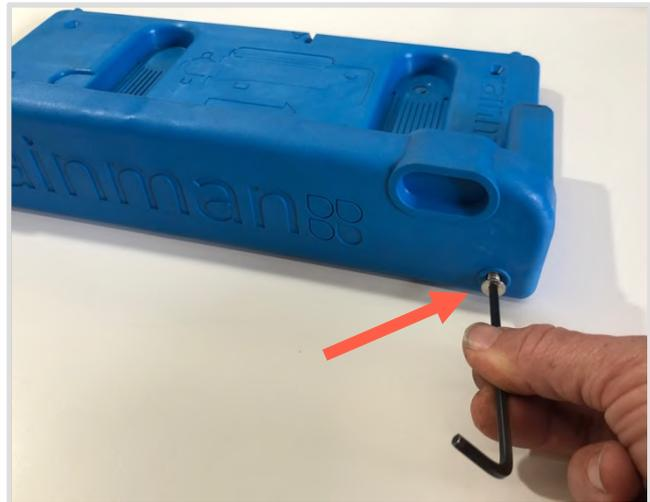
2. Fasten the mounting seat to a level surface using all four holes. Use the self-tapping screws provided, or your choice of alternate fastener.
